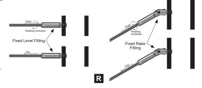
2. Feed the cable through any Pass Through Newels toward the Tensioner Fitting at the opposite end of the run. Mark the cable at the score mark on the body of the fitting. Cut the cable at this mark (S).
