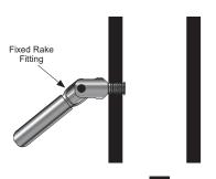
To install the Tensioner Rake Fittings, drive the machine threads of the hinged portion of the fitting into the hole on the Rake Up Newel. Using the articulating portion of the fitting as a lever to rotate the threads of the fitting into the newel (M). Tip: Using a 6"-8" piece of 3/4" PVC tube over the articulating portion may make this task easier.
