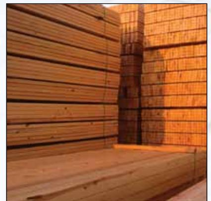
All of our wood is treated with mold inhibitor as well as preservative. We also provide wood that is dried after treatment via two propane powered dry kilns. All dried-after-treatment material is covered with a weather-resistant wrapping.
