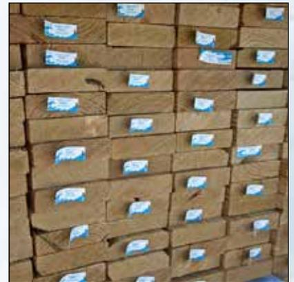
Samples taken from each charge are analyzed to ensure consistent quality of the treatment. Tarpred trucks, indoor storage, multiple inspections, automated handling equipment, and consistent treatment practices are all measures that ensure customers get bright, freshly processed material on every order.
