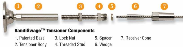
Figure AY. HandiSwage™ Tensioner components.
