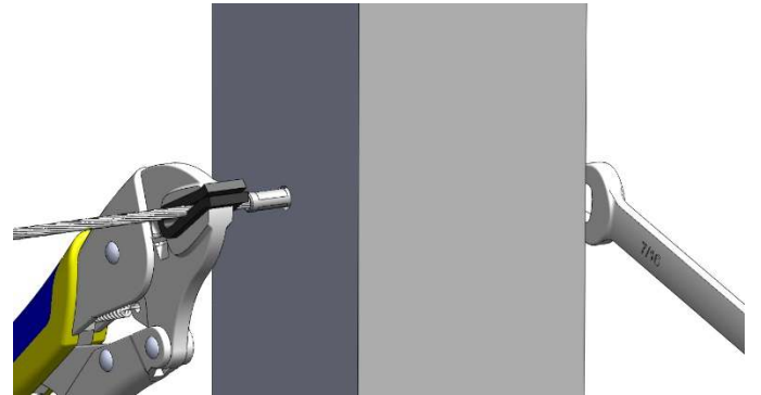
Figure V. Option two (2) is to use a cable grip pad to hold the cable just outside the post while tightening the nut.
