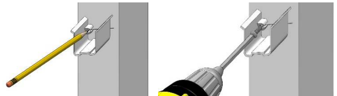
Figure AG. Mark the saddle bracket hole locations and attach with self-drilling screws.
