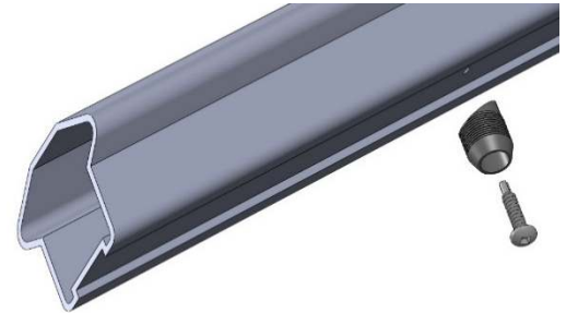
Figure AL. Install the stabilizer and support block connectors using a 1" self-drilling screw.
