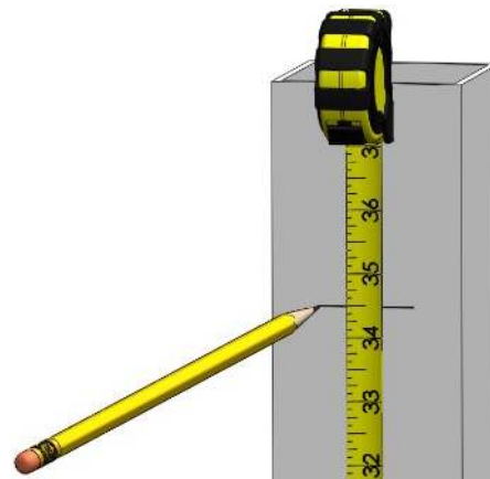
Figure D. Measure up 34-1/2" for a 36" rail height from the mounting surface and mark a level, horizontal line.
