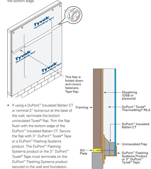
If using the termination ledge, remove the uninsulated Tyvek<sup>®</sup> flap at the bottom and secure to the termination strip with a DuPont<sup>™</sup> Flashing Systems product or DuPont<sup>™</sup> Tyvek<sup>®</sup> Tape.
