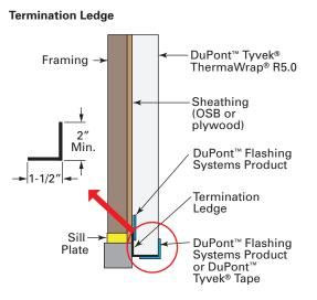
If a termination accessory is not used, seal the flap at the bottom of the wall with a DuPont<sup>™</sup> Flashing Systems product, DuPont<sup>™</sup> Tyvek<sup>®</sup> Tape, or DuPont<sup>™</sup> Residential sealant. The uninsulated Tyvek<sup>®</sup> flap should cover the bottom edge of insulation before turning down onto the foundation.
